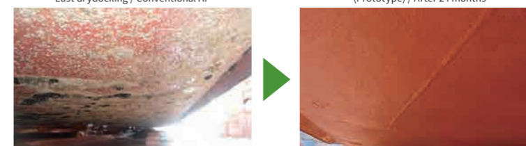
SEAFLO NEO M1 PLUS can reduce a risk of barnacle fouling in static condition and low activity operation.
