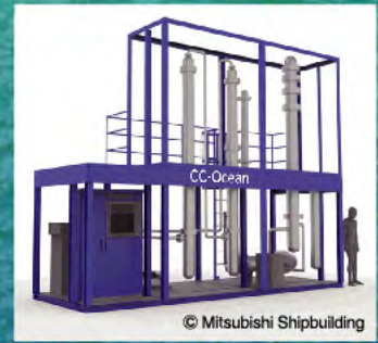
© Mitsubishi Shipbuilding Conceptual drawing of the CO 2 recovery demo plant
